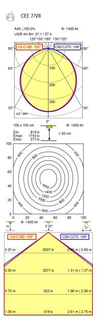
light source LED work equipment electronic transformer connected load 100-240 V, 50/60 Hz; secondary 24 V, DC power consumption env. 23 W luminous flux approx. 1.400 lm luminous efficiency approx. 74 lm/W light type/-color cold white colour temperatur approx. 5.000 K
